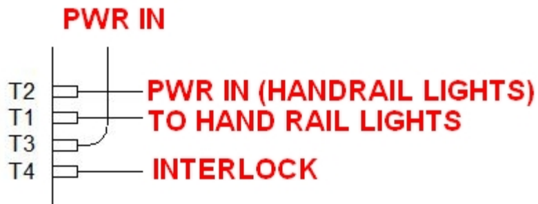
FIGURE 4: PREVIOUS TERMINAL ORIENTATION
