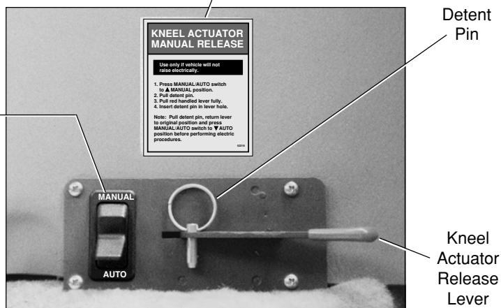
Kneel Actuator Manual Release Instructions Decal #52215
